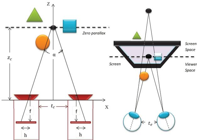
**Fig. 2** A virtual camera setup with parallel sensor-shift (left) and the corresponding reconstruction of stereoscopic 3D scene
